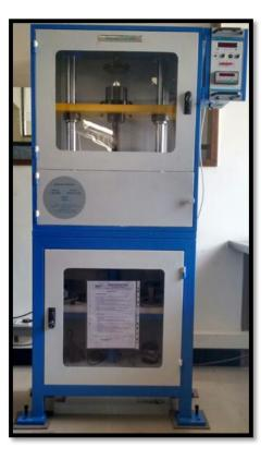
Spring Testing System (Manual Version)
