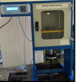
Spring Testing System (Manual Version Table Top)
